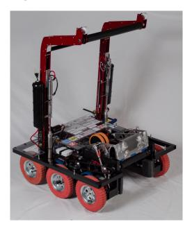
If the lower cylinder extends, the arms move up to raise the portcullis. If both cylinders are retracted, the robot will lower ramps on the Cheval-de-Frise.
