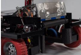
The boulder, after being held by the intake roller while the shooter reaches desired rpm, is launched by two orange BaneBot wheels and an aluminum flywheel. These are driven by a 3:1 planetary gearbox on a 775 Pro motor.
