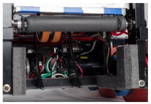
A line break sensor tells the intake roller to stop when the ball is in the desired position.
