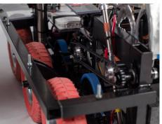
"Knight Mare" drives on a custom West Coast drive train utilizing 10 wheels: 6 outer eight inch diameter pneumatic wheels and 4 inner five
